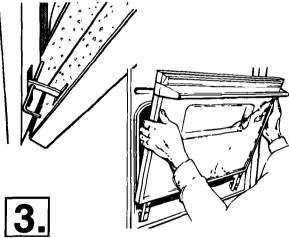
Self-cleaning ovens: Insert a nail (or equivalent, 5/32" diameter item) into the hole in each of the hinges. Close the door as far as possible. Lift the oven door off of the hinges. Set aside.
